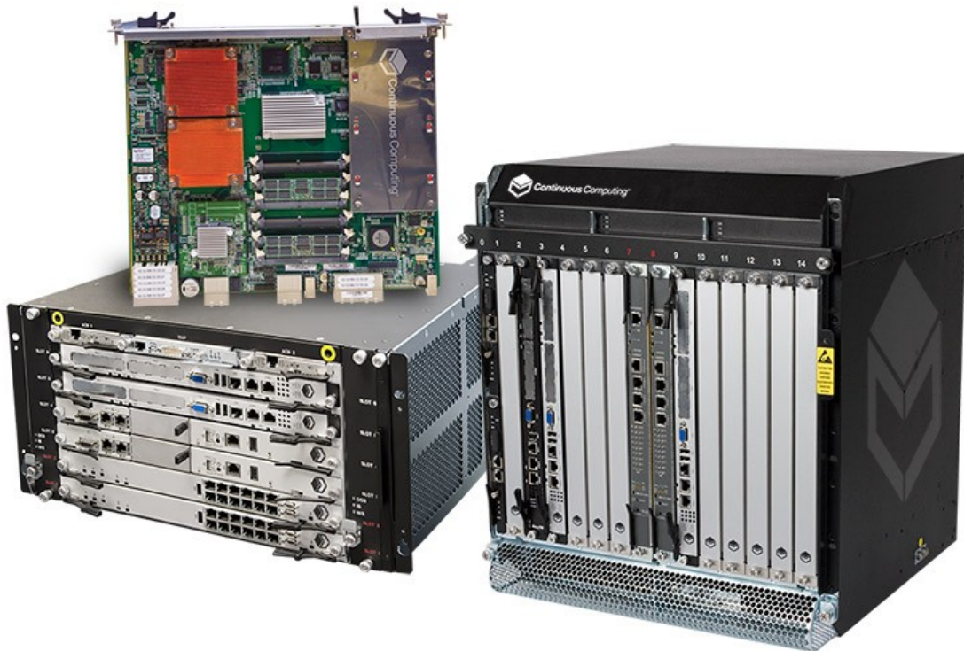
Figure 5.1: ATCA crates and boards
