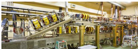
Figure 8: Photograph of the new thermionic electron gun beam line.
