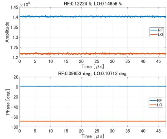
Figure 7: Amplitude and phase stabilities of RF and LO signal measured with simultaneous direct sampling from RF-LO combined signal.
