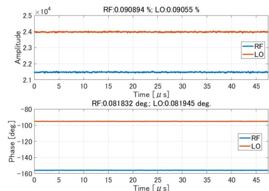
Figure 4: Amplitude and phase stabilities of RF and LO signal measured with simultaneous direct sampling.
