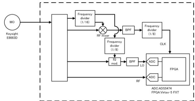
Figure 2: Experimental setup of RF-LO simultaneous measurement.
