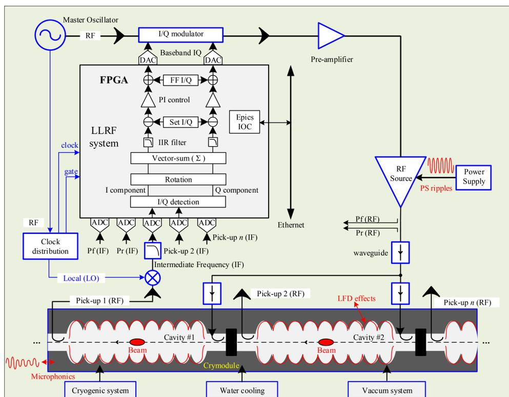
Figure 1: Schematic of the LLRF system and the typical disturbance sources.
