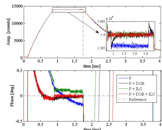
Figure 5: Comparison of P control (blue), “P+DOB” control (black), “P+ILC” control (green) and “P+DOB+ILC” control.
