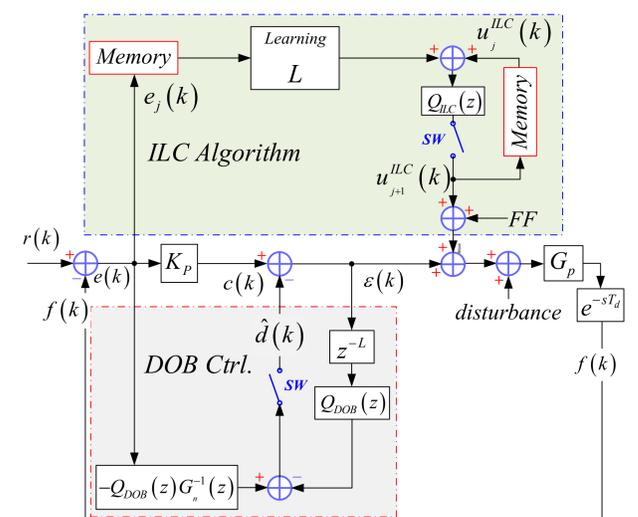
Figure 4: Combined control algorithm including P control, ILC algorithm and DOB control.
