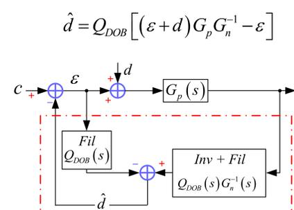
Figure 3: DOB control with Q-filter.
