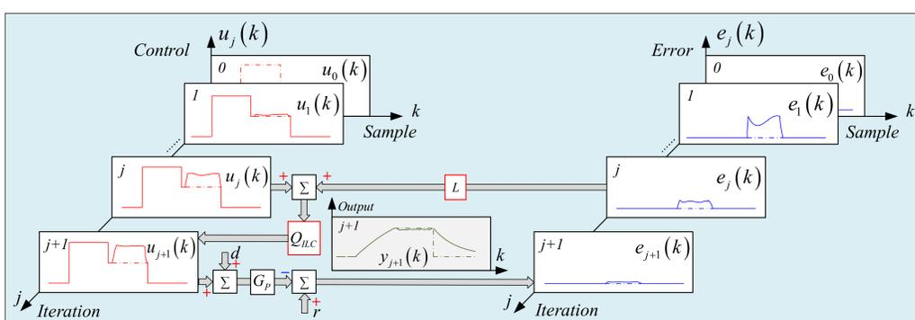
Figure 2: Learning process of ILC algorithm
