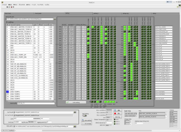
Figure 5: Interlock Application on cRIO.
