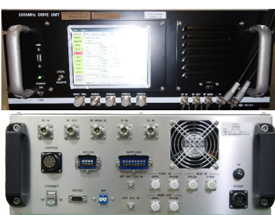
Front/rear panel of LLRF control unit
