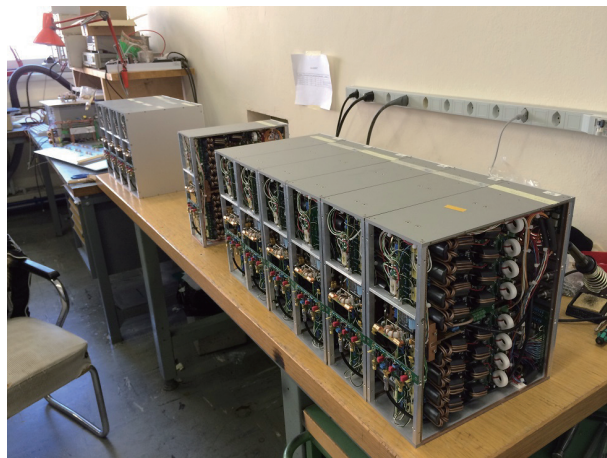
Figure 2: Solid state amplifiers for CERN PSB FT3L cavities.
