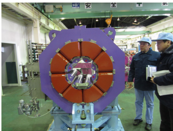
Figure 5: Fabricated octupole magnet with field gradient of 800\text{ T/m}^3 .
