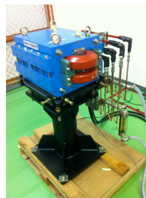
Figure 3: Kicker magnet made of 0.35 mm laminated silicon steel plates.
