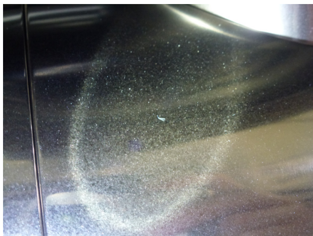
Figure 6: Photograph of a dust on the cathode ball.
