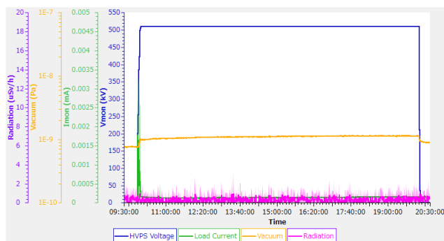
Figure 8: Trend graph of 500 kV high voltage holding test. There is no trip or discharge problem during 10 hours.
