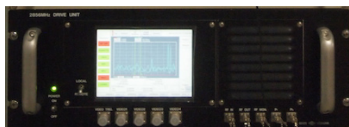
Figure 5 b): The photograph of a new Klystron Drive System.
