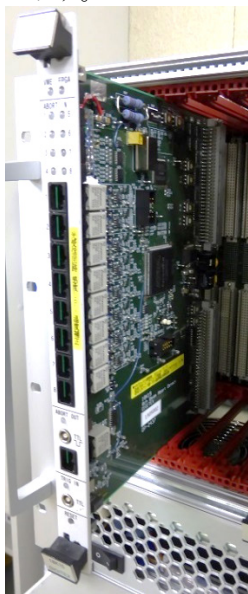
Figure 2: 8ch beam abort optical input module (18K15).
