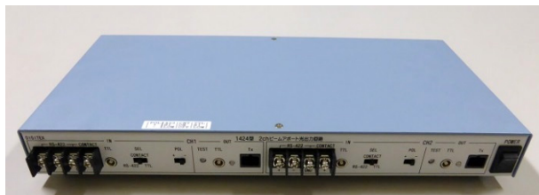
Figure1: 2ch beam abort optical output module (1424).
