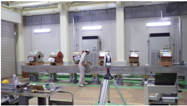
Figure 6: A Support Under Measurement by AT-401.
