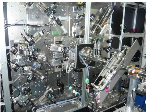
Figure 4: Beam size monitor at ATF2-IP.
