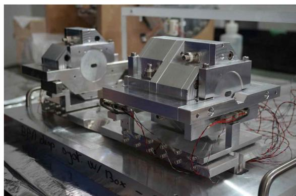
Figure 7: Cavity BPM on piezo mover.
