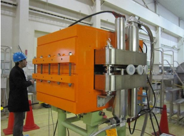
Figure 5: HTS switching magnet.
