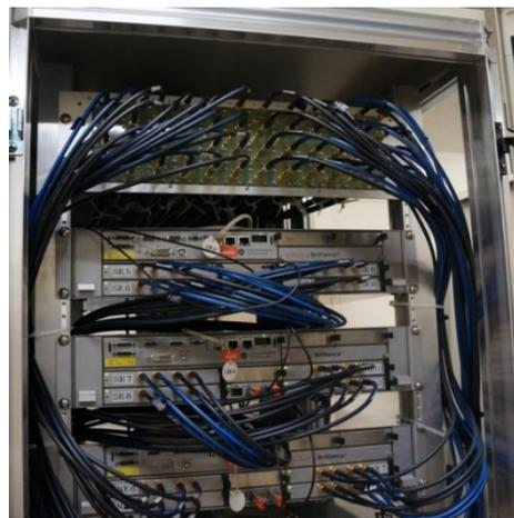
Figure 4: A part of the new beam position circuits installed into the standard 19 inch rack. Low loss 8D-size cable connects between each electrode and the panel on the upper part of the rack. A 2U-height box contains four detection circuits.
