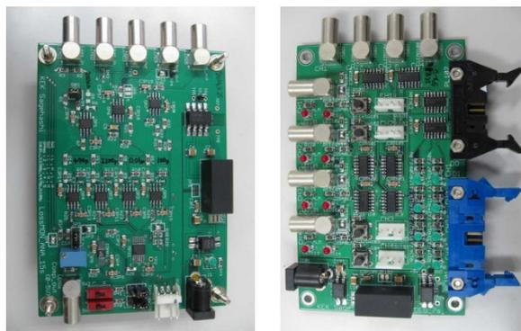
Figure 3: Integrator comparator & latch circuit board.
