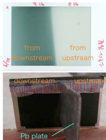
Figure 3: Setup with a lead plate for direction measurement.
