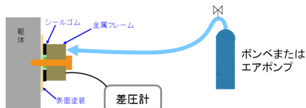
Figure 12: Pressurization method to test the sealing of frame and a concrete wall.
