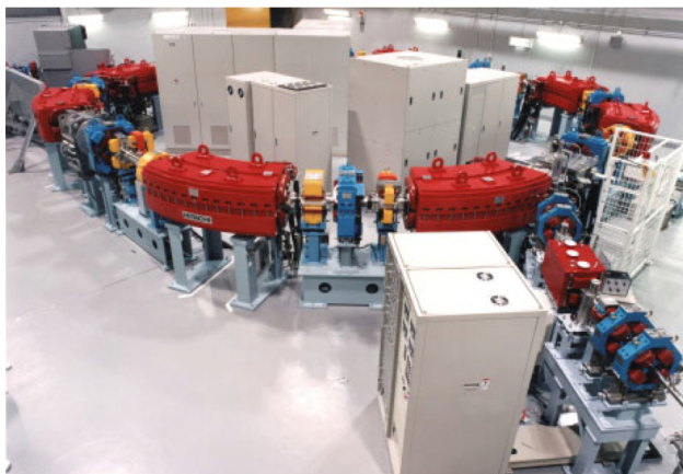
Figure 4: Panoramic view of the synchrotron. Tandem beam is injected along the beam line at the lower right.
