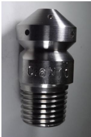
Figure 6 : High pressure rinsing nozzle.
