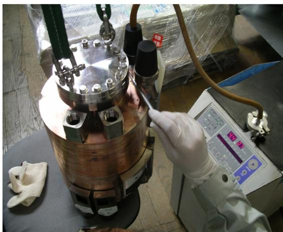
Figure 1: Fixing of the water leakage from a silver brazing part between copper and stainless steel in a water cooling channel using liquid gasket.
