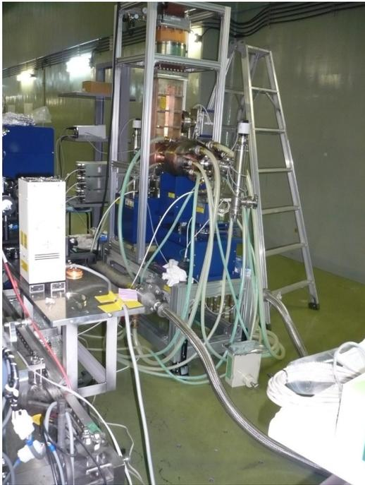
Figure 4: L-band RF gun under high power testing at KEK-STF.
