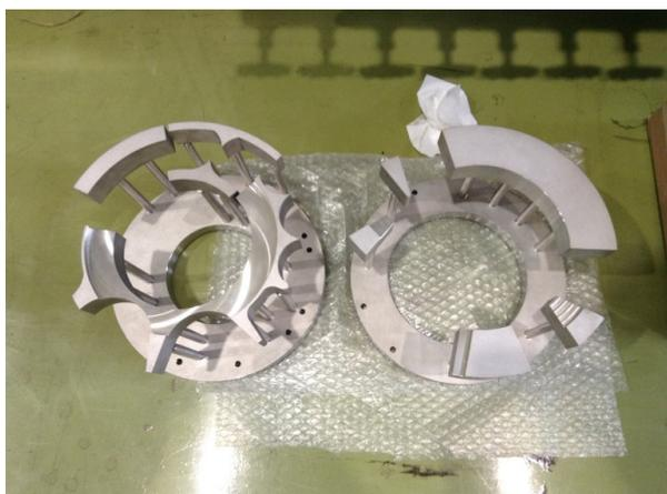
Figure 2: Special jigs for tuning the frequency and the electric field balance between the half and the full cells of the RF gun.
