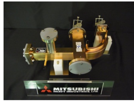
Figure 2: Completed E bend.
