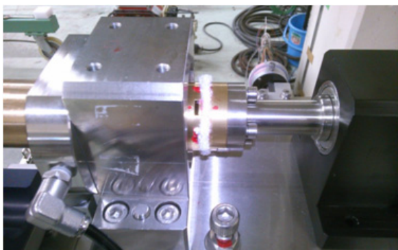
Figure 11: The improvement of the driven side coupling.
