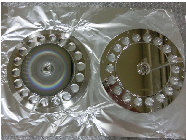
Figure 7: Old and new anode disks, Left: old (15years used), Right: new.
