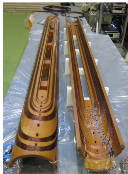
Figure 8: Two 2-m long coils after curing.
