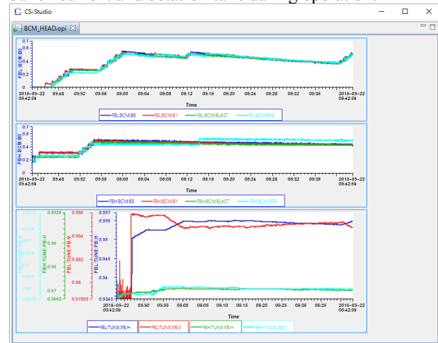
Figure 4: Example of measured bunch current (upper) and the betatron tune with PLL method (lower).
