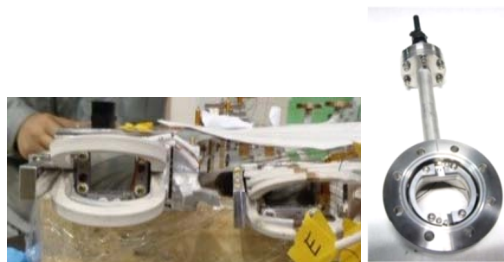
Figure 4: Examples of slit enhancements. Left figure shows the enhancement of magnetic channel from 15mmX15mm to 33mmX30mm. And right figure is for slit “B” in Figure 3 from 30mmX24mm to 36mmX30mm.
