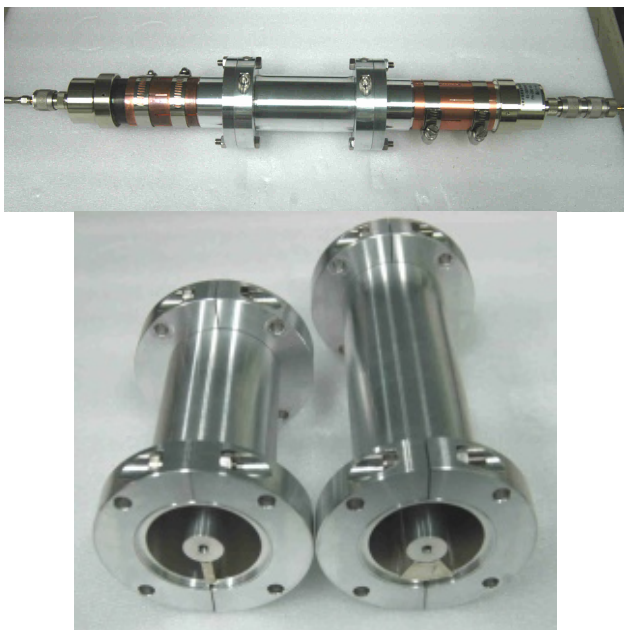
Figure 1: CWG transmission model (top). CWG with parallel connecting plate (bottom left) and CWG with radial connecting plate (bottom right).
