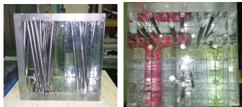
Figure 4: The acrylic phantom which contains steel rods. The diameters of rods are from 6 to 10 mm.
