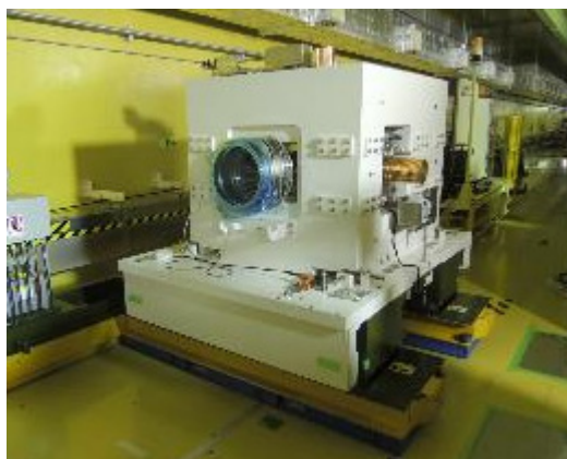
Figure 4: A new collimator with movable blocks. The installation was postponed to summer 2018.
