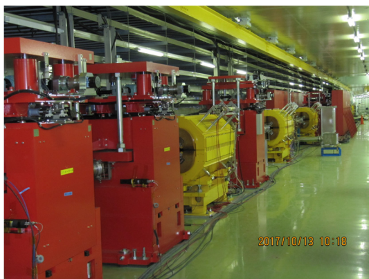
Figure 5: Collimators (in red) after the rearrangement.
