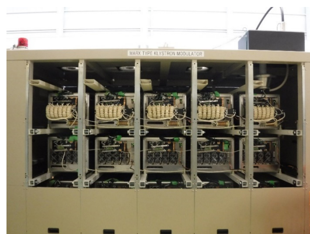
Figure 8: Photograph of the Chopper-type Marx units with common mode filter.
