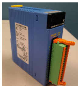
Figure 1: F3HA06 - high-speed data acquisition module.
