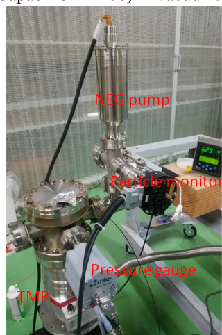
Figure 5: Measurement system of dust of NEG pump (CapaciTorr HV200) in vacuum.
