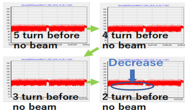
Figure 4: Bunch oscillation monitor signals in a damaged event.
