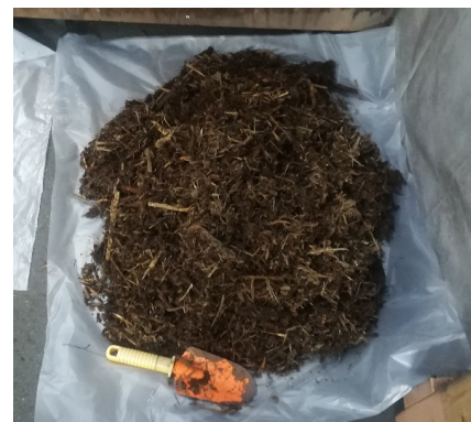
(b) HASClay covered with wood chips.
