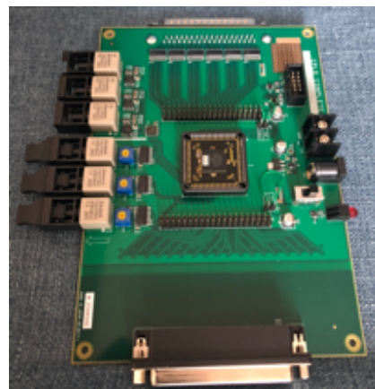
Figure 11: Adder board we have designed for the beam experiment using one half-arc of MR.
