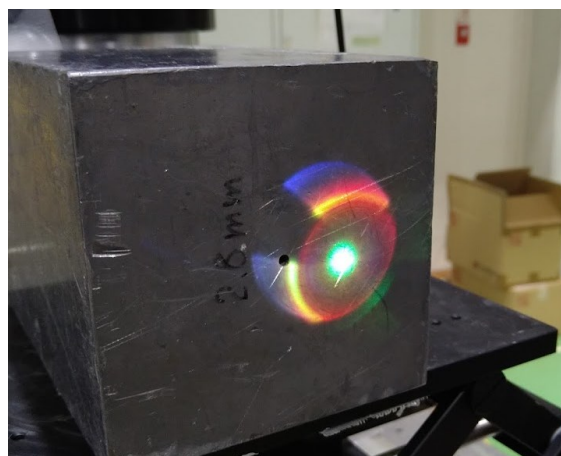
Figure 6: Photo of FEL beam on the collimator when the collimator position was optimized to have highest flux of gamma ray observed by an NaI scintillation detector.
