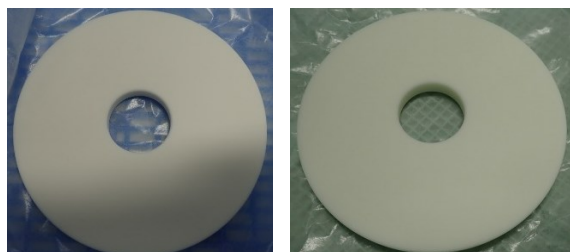
Figure 21: Ceramic samples (AO479U and AO479B from left to right) for Dielectric loss tangent measurement.
