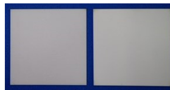
Figure 17: Ceramic samples (AO479U and AO479B from left to right) for relative permittivity and Dielectric loss tangent measurement.
