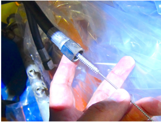
Figure 5: Cleaning the inside of a hose with a special brush.
