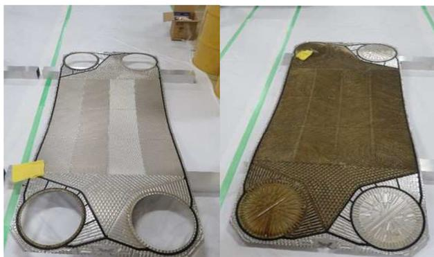
Figure 6: The exchanger plates. The left picture shows the primary loop side, and the right picture shows the secondary loop side.
