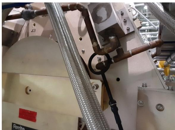
Figure 5: A loop antenna we used and largest leakage source in the circulator.
