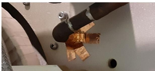
Figure 7: Circulator hole sealed by copper tape.
