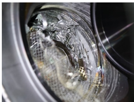
Figure 3: Damaged TMP used for the extraction chamber of the RIKEN 28 GHz ECR ion source.
