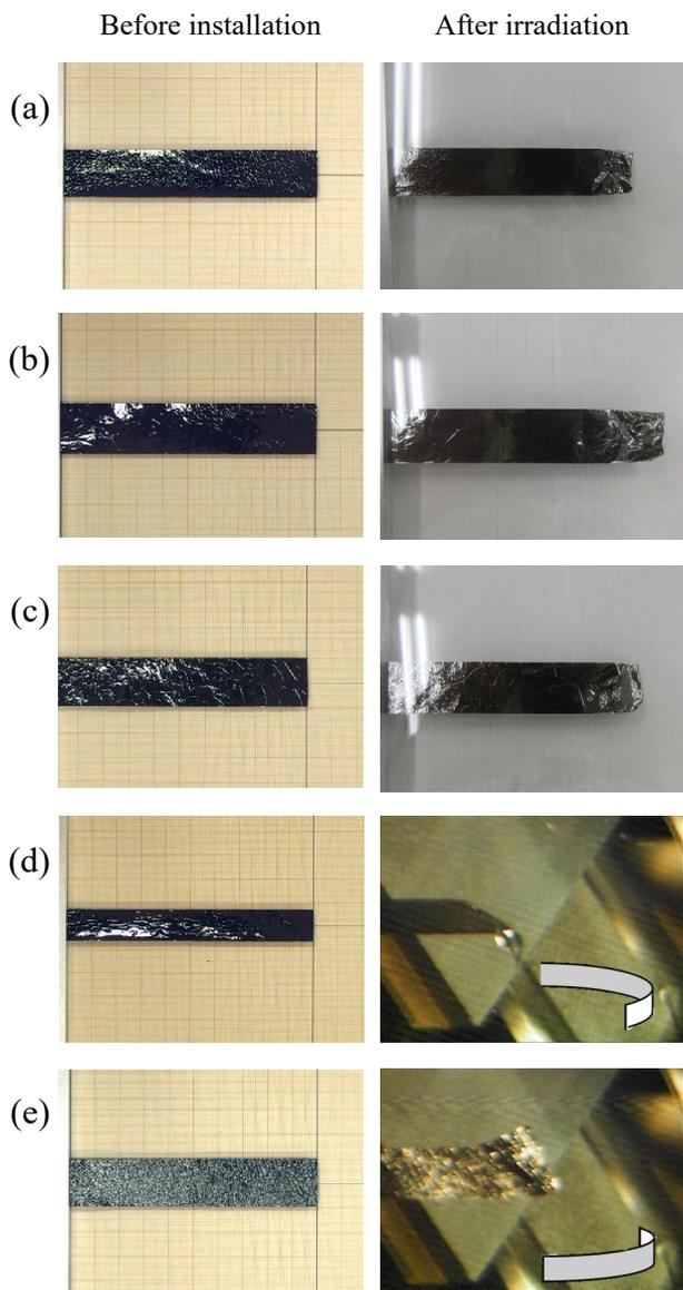
Figure 2: Pictures of the foils before installation and after irradiation at 2020-2021.
