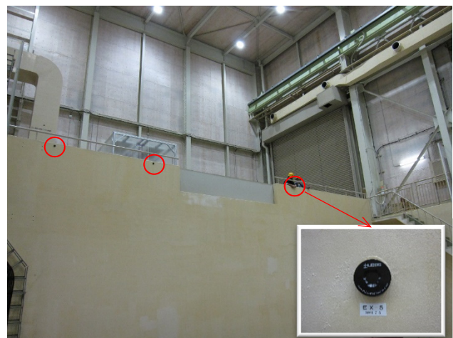
Figure 4: Target holders in the experimental hall.
