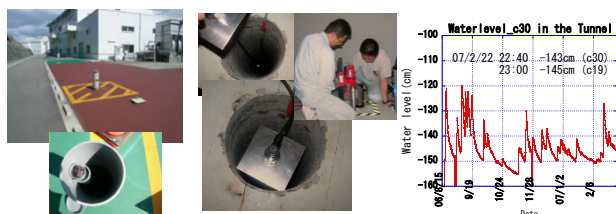
(a)Outside well (b)Inside well (c)Water level of (b) Figure 11: Measuring water levels in the wells.
