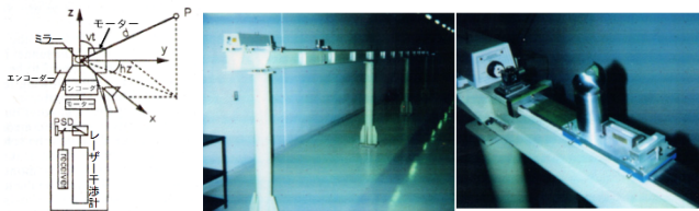
(a)Laser Tracker (b)Laser interferometer HP5527A on the 20m-long rail
