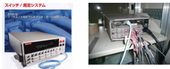
(a)Front panel (b)Rear panel Figure 6: Data acquisition system Keithley 2701.
