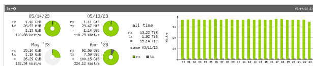
Figure 2: Example of network traffic monitoring and recording with vnstat.
