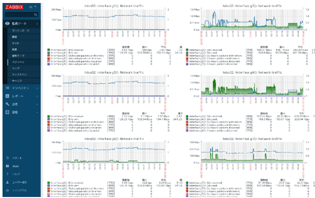
Figure 6: Example of Zabbix screen for monitoring network smart switch information.
