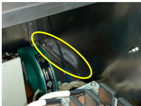
Figure 10: Photograph of the white deposition observed at the Al plate.
