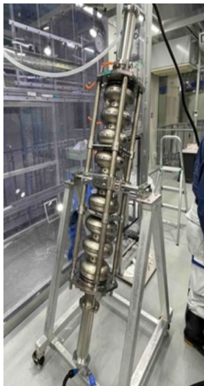
Figure 5: Ultrasonic cleaning of the cavity with two oscillators.
