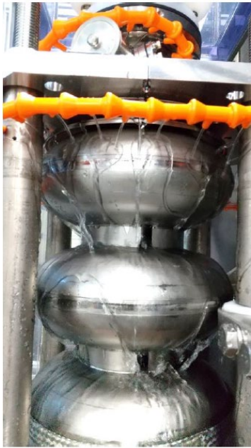
Figure 4: Cavity cooling with pure water.
