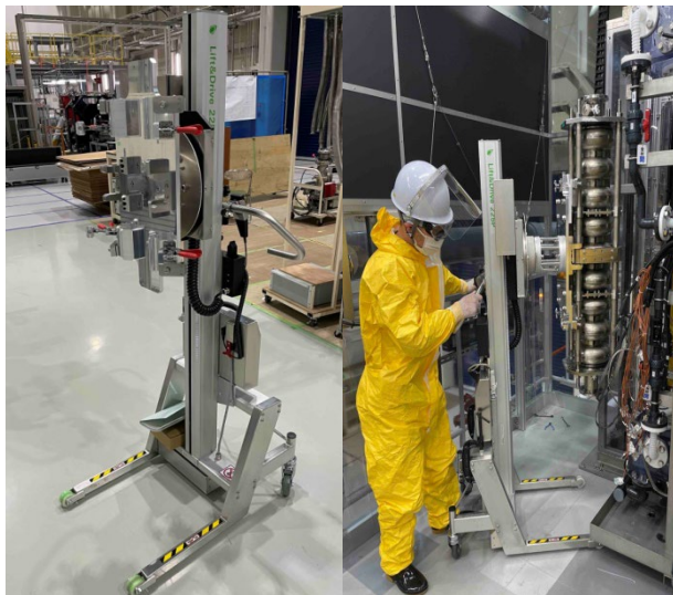
Figure 1: Electric lifter for cavity transport (left) and installation of 9-cell cavity in the EP bed (right).
