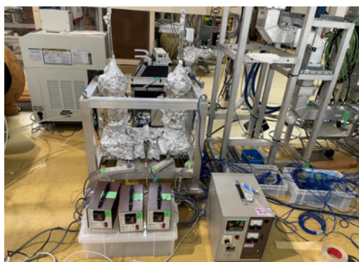
Figure 3: Configuration for the coupler baking process.
