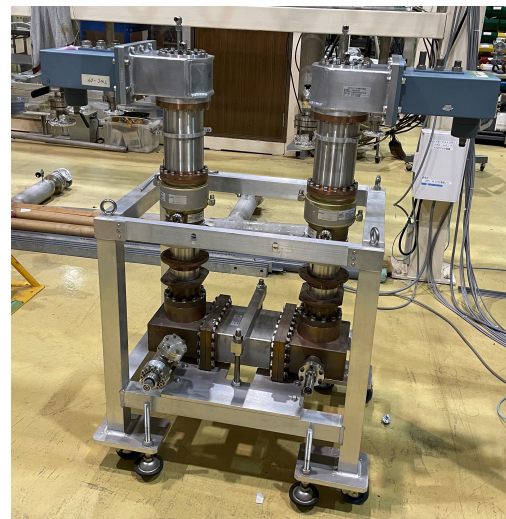
Figure 1: cERL injector prototype coupler test stand.
